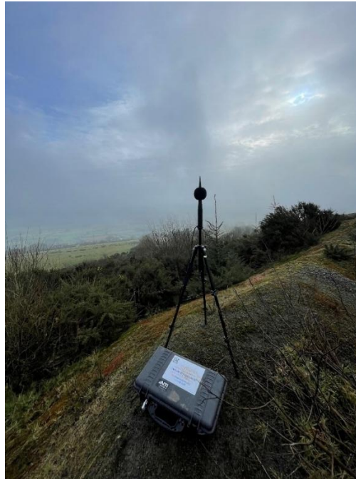
Figure 11.3: Noise measurement setup.
